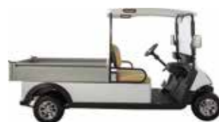
-Shuttle A/B aluminum cargo box Aluminum cargo box size:1478*1145*270mm
