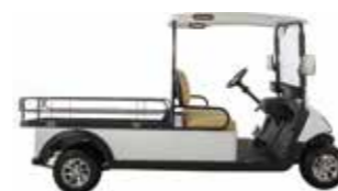
-Shuttle A/B cargo deck Cargo box size:1735*1160*350mm
