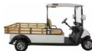
-Shuttle A/B wooden cargo box Wooden cargo box size:1505*1180*310mm
